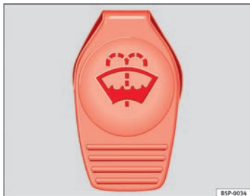
Fig. 166 In the engine compartment: Cap of windscreen washer fluid reservoir.
