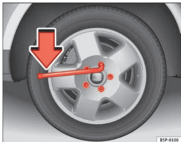
Fig. 176 Changing the wheel: loosen the wheel bolts
