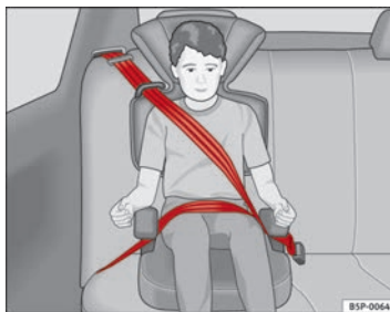
Fig. 30 Forward-facing child seat installed on rear seat.
