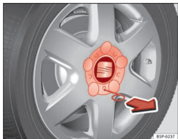
Fig. 175 Changing the wheel: Removing a hub cap
