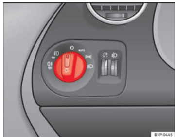
Fig. 73 Detailed view of the dash panel: lights, fog lights and rear fog light switch
