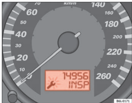
Fig. 38 Service interval display
