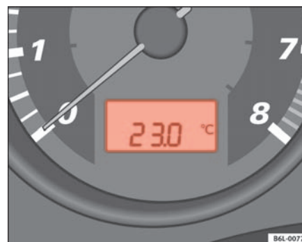
Fig. 35 Digital screen on the instrument panel: outside temperature display
