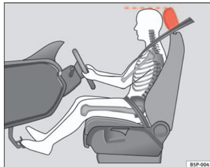
Fig. 2 Proper head restraint position for driver
