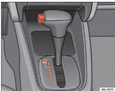
Fig. 101 Section of centre console: selector lever on cars with an automatic gearbox
