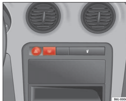
Fig. 59 Detail of the dash panel: Hazard warning light switch
