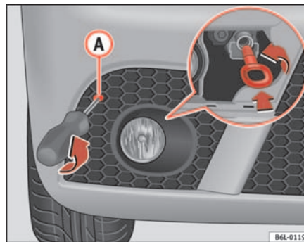
Fig. 171 Towing eye at the front of the vehicle
