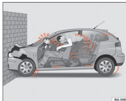
Fig. 7 The vehicle with unbelted occupants strikes the wall.
