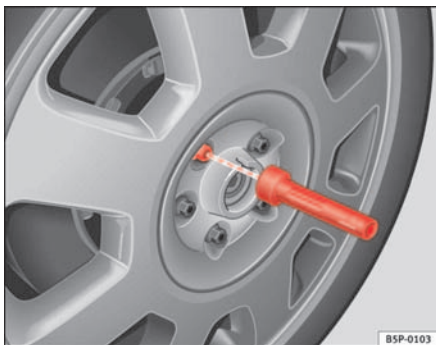
Fig. 144 Wheel change: Hexagon socket in screwdriver handle to turn the wheel bolts after they have been loosened
