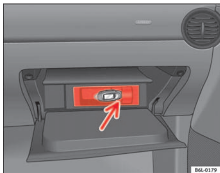
Fig. 88 USB* connection in the passenger side glove compartment
