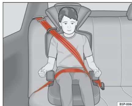
Fig. 28 Forward-facing child seat installed on rear seat.
