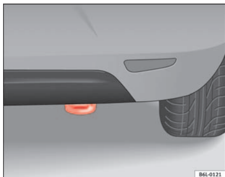
Fig. 175 Rear towing ring
