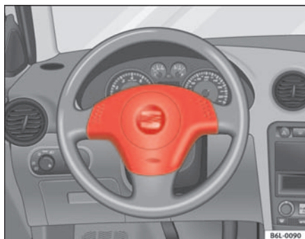
Fig. 16 Driver airbag located in steering wheel
