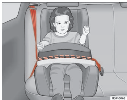
Fig. 27 A category 1 forward-facing child seat fitted on the rear seat.
