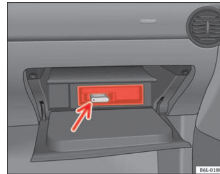
Fig. 87 iPod connection in the passenger side glove compartment
