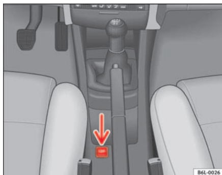
Fig. 98 Detail of the centre console: ESP button
