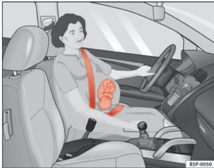
Fig. 14 Positioning seat belts during pregnancy
