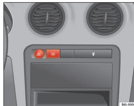
Fig. 58 Instrument panel: rear window heater switch ▶
