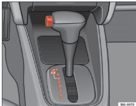
Fig. 102 Section of centre console: selector lever on cars with an automatic gearbox
