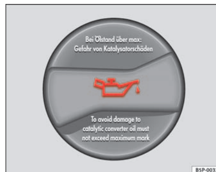
Fig. 128 In the engine compartment: Engine oil filler cap
