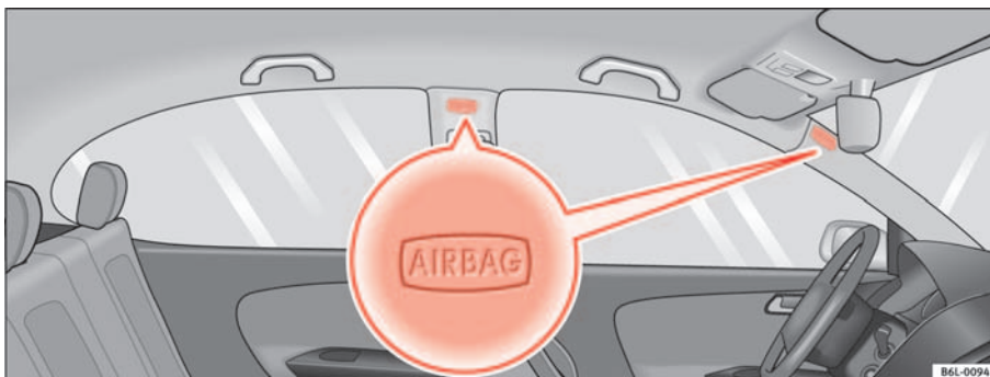
Fig. 22 Location of left curtain airbag
