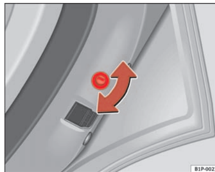
Fig. 44 Child safety lock on the right-hand side door
