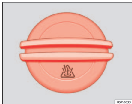
Fig. 129 In the engine compartment: Coolant expansion tank cap
