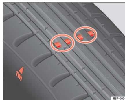
Fig. 134 Tyre tread wear indicators
