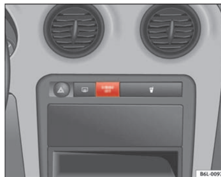
Fig. 25 Warning lamp for deactivated passenger airbag in centre console
