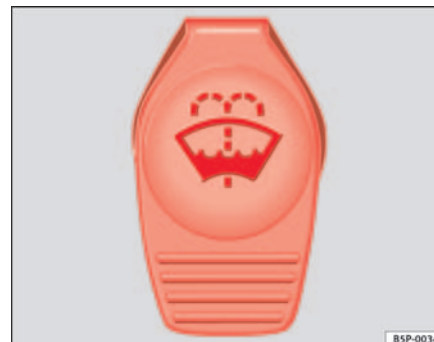
Fig. 130 In the engine compartment: Cap of windscreen washer fluid reservoir.
