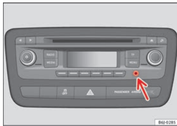
Fig. 94 Centre console: AUX Connection.
