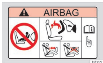
Fig. 15 Sun visor on the front passenger's side: airbag sticker.
