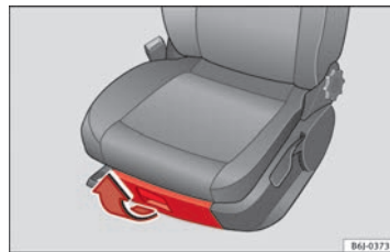
Fig. 86 Storage compartment under the front passenger seat.
