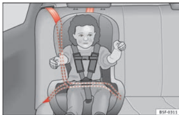
Fig. 27 A category 1 forward-facing child seat fitted on the rear seat
