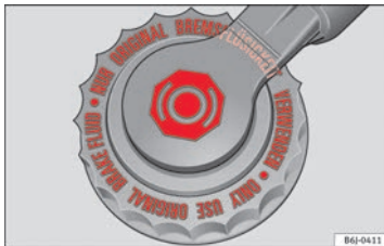
Fig. 144 In the engine compartment: Brake fluid reservoir cover.
