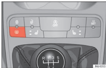
Fig. 64 Centre console: heated rear window switch.
