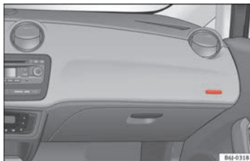
Fig. 18 Front passenger airbag located in dash panel.
