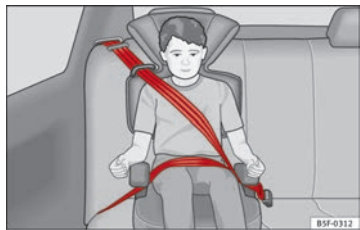
Fig. 28 Forward-facing child seat installed on rear seat
