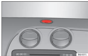
Fig. 84 Mounting bracket for navigator on dash panel.
