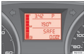
Fig. 38 Digital display: Gearbox lever position for automatic gearbox.
