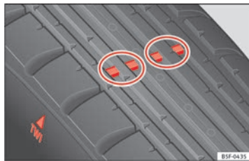
Fig. 145 Tyre tread wear indicators.
