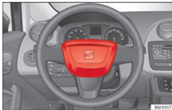
Fig. 17 Driver airbag located in steering wheel.
