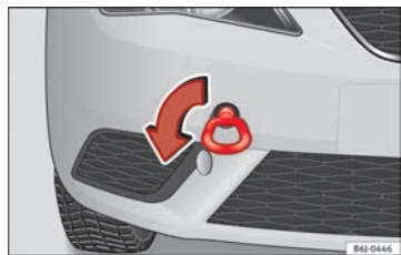
Fig. 191 Fitting the towline anchorage to the front of the vehicle.
