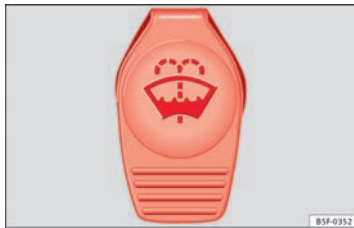
Fig. 140 In the engine compartment: Cap of windscreen washer fluid reservoir
