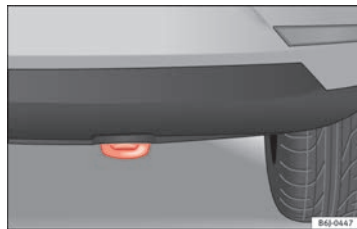
Fig. 192 Rear towline anchorage.
