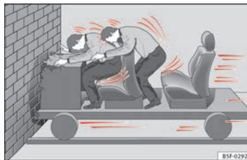
Fig. 7 The vehicle hits the wall: the vehicle occupants are not wearing seat belts
