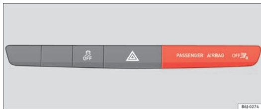
Fig. 22 Centre side of dash panel: control lamp for deactivated front passenger airbag in centre console.
