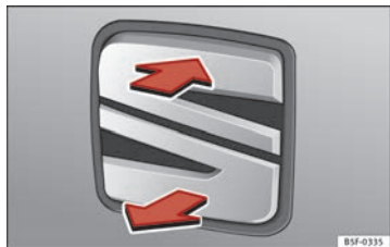
Fig. 52 Rear lid: opening from the outside.
