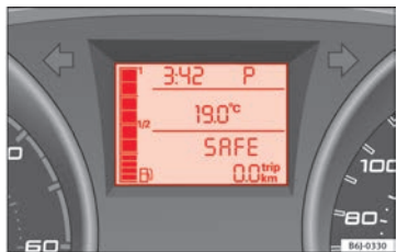
Fig. 123 Automatic gearbox: instrument panel display.
