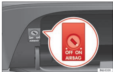
Fig. 21 In the glove compartment: switch for activating and deactivating the front passenger airbag.
