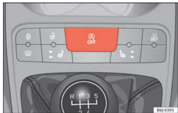
Fig. 114 The Start-Stop function button.
