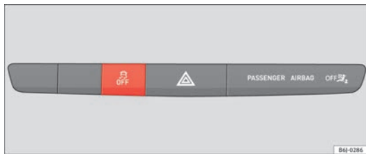
Fig. 112 Detailed view of the dash panel: ESC switch.
