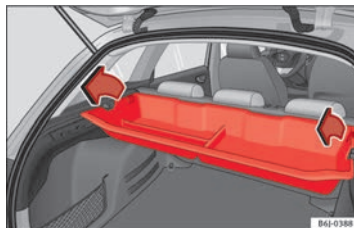
Fig. 101 Luggage compartment: removing storage compartment.
