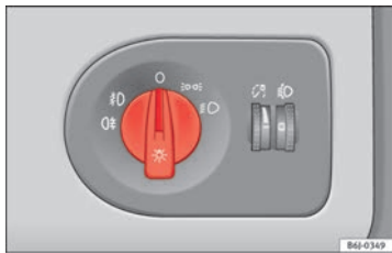
Fig. 60 Detailed view of the dash panel: lights, fog lights and rear fog light switch.
