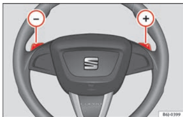
Fig. 122 Steering wheel with paddle levers for automatic gearbox.
