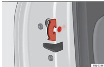
Fig. 47 Childproof lock on the left hand side door.
