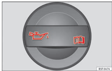
Fig. 138 In the engine compartment: Engine oil filler cap.
