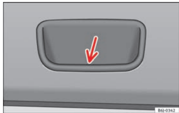
Fig. 53 Close-up of the inside trim of the rear lid: hand grip
