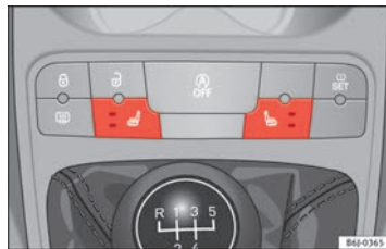
Fig. 78 Front seat heating switch.
