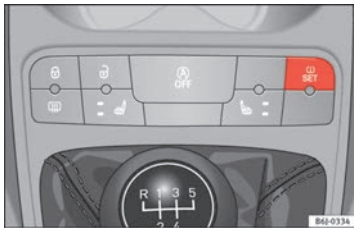
Fig. 41 Centre console: tyre monitor system button. ▶
