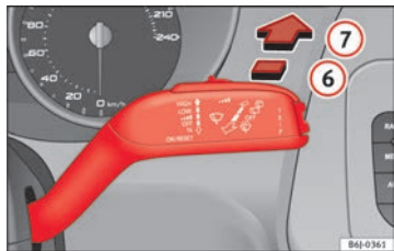
Fig. 72 Windscreen wiper lever: window wiper.
