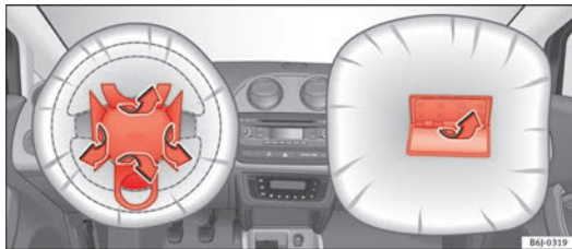
Fig. 20 Airbag covers reacting when the front airbags are triggered.
