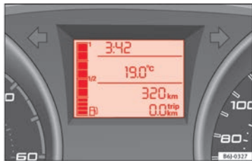
Fig. 35 Instrument panel: fuel gauge
