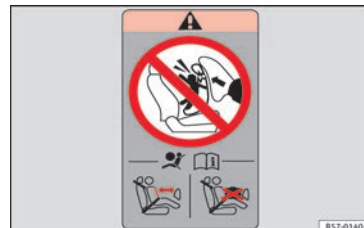
Fig. 21 On the rear frame of the passenger side door: airbag sticker.
