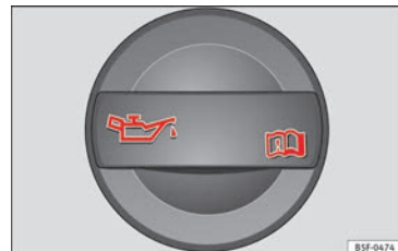
Fig. 47 In the engine compartment: Engine oil filler cap.
