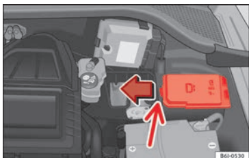
Fig. 52 In the engine compartment: fuse box cover.
