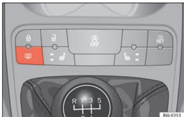
Fig. 120 Centre console: heated rear window switch.
