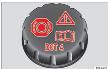
Fig. 49 Engine compartment: brake fluid reservoir cap.
