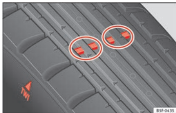
Fig. 157 Tyre tread wear indicators.
