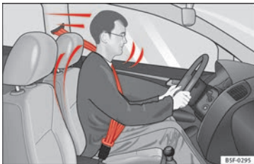
Fig. 73 Drivers with properly worn seat belts will not be thrown forward in the event of sudden braking.
