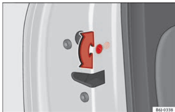
Fig. 112 Childproof lock on the left hand side door.
