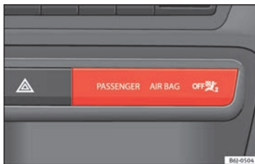
Fig. 79 Centre side of dash panel: control lamp for deactivated front passenger airbag in centre console.
