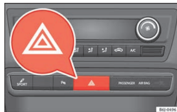
Fig. 29 Dash panel: switch for hazard warning lights.
