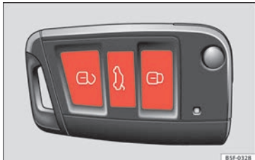
Fig. 1 Remote control key: buttons.
