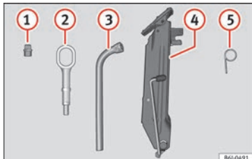
Fig. 55 Underneath the floor panel of the luggage compartment: vehicle tool kit.
