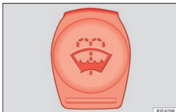
Fig. 50 In the engine compartment: windscreen washer reservoir top.
