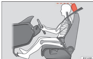
Fig. 69 Correct head restraint position for the driver.
