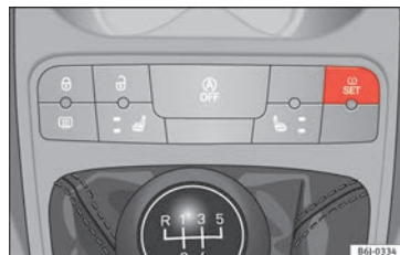
Fig. 159 Centre console: tyre monitoring system button.
