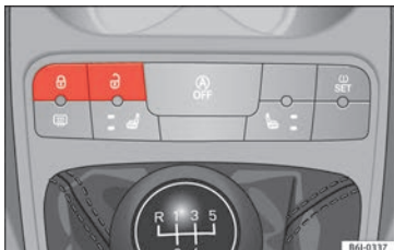
Fig. 2 Centre console: Central lock buttons.
