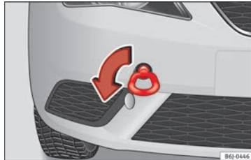
Fig. 61 Right side of the front bumper: Towing ring.
