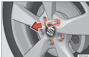
Fig. 56 Wheel: wheel bolts with caps.
