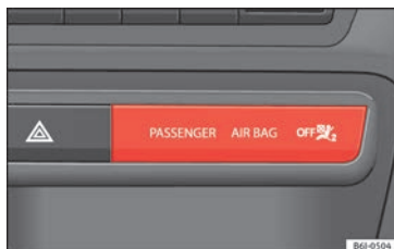
Fig. 41 Warning lamp for disabling the front passenger airbag.
