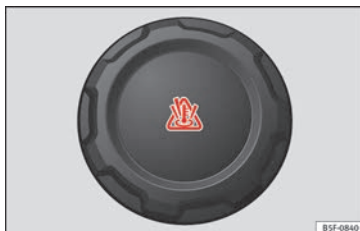
Fig. 48 Engine compartment: coolant expansion tank cap.
